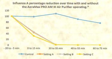
\*Results represent the average of n=3 runs. Device settings A: ionizer ON and filter low speed; device setting B: ionizer off and filter at low speed; device setting C ionizer of and filter at high speed.
